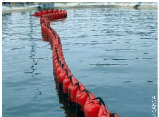
Boom deployed on the water surface.
