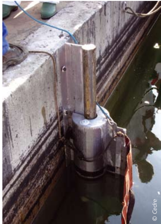
Boom mooring arrangements and tidal compensators: slide rail fixed to the quay (right) or sliding shackle on a ballasted rope (left).
