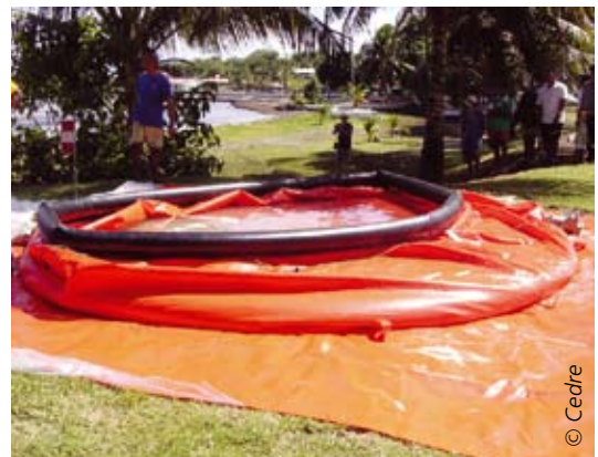
A flexible self-erecting tank.
