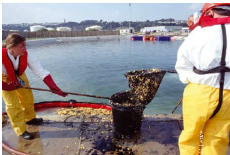
Recovery of heavy fuel oil on the water surface using bulk sorbents and landing nets during an exercise at Cedre's technical facilities.
