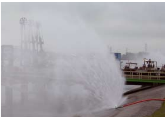
Water curtain sprayed by water shields in series.
