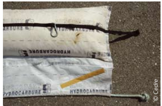
Sorbent boom with ballasted skirt and connectors positioned for overlapping connection.
