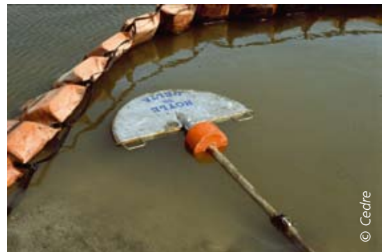
Lightweight flat suction head for floating pollutant.
